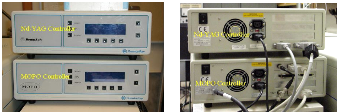
Figure 6: Top left shows the front of the Nd-YAG and MOPO. Top right shows the back of the Nd-YAG and MOPO controller where the ON/OFF switches are located.
