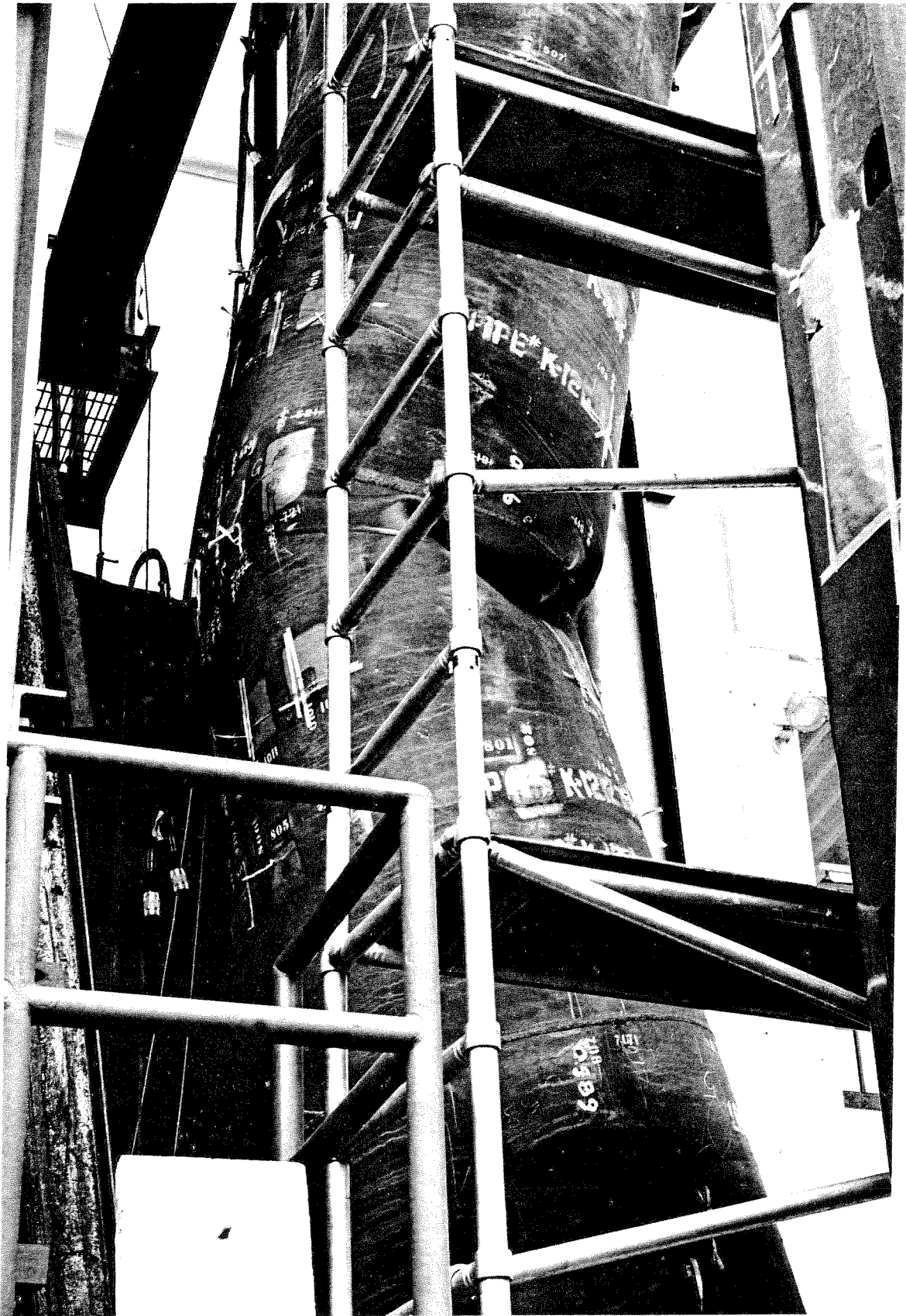
FIG. 42 SPECIMEN NO. 7 SIDE VIEW AFTER POST-BUCKLING TEST
