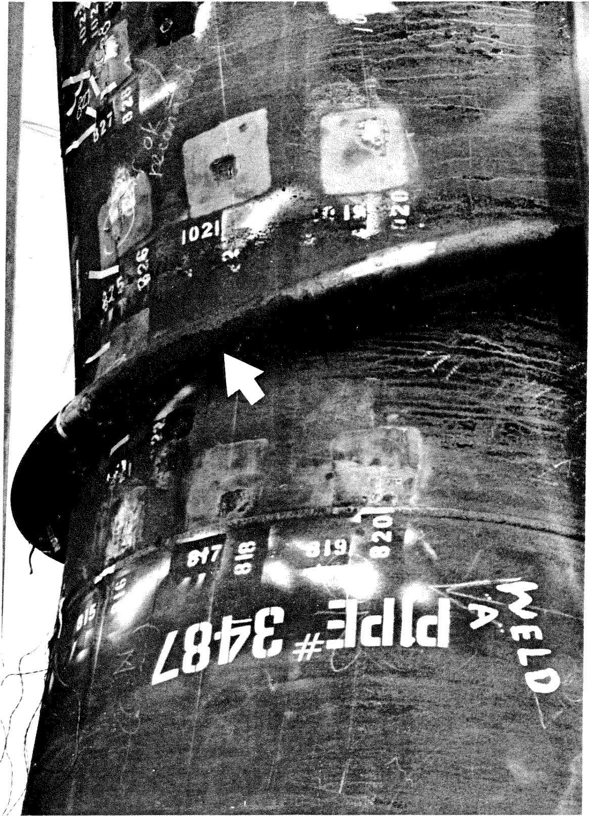
FIG. 15 SPECIMEN NO.2 -AFTER POST-BUCKLING TEST- COMPRESSION FACE
