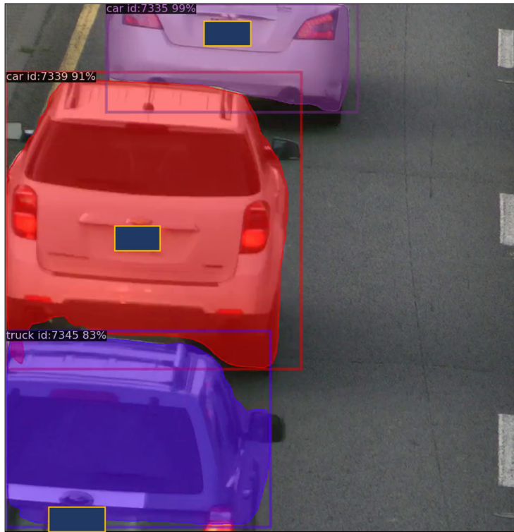
Figure 143 – Auto Crop of Images with Confidence Level by Machine Vision
