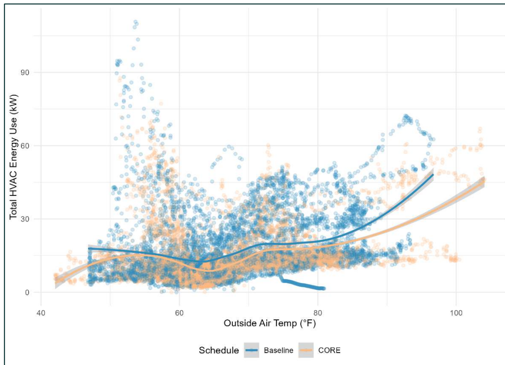
Figure 55: HVAC heating, cooling, and fan energy consumption vs. OAT for combined AHU 1 and AHU 2—MOB-3.
