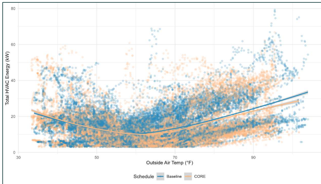
Figure 36: HVAC heating, cooling, and fan energy consumption vs. OAT for combined RTU 1 and RTU 2/3—MOB-2.
