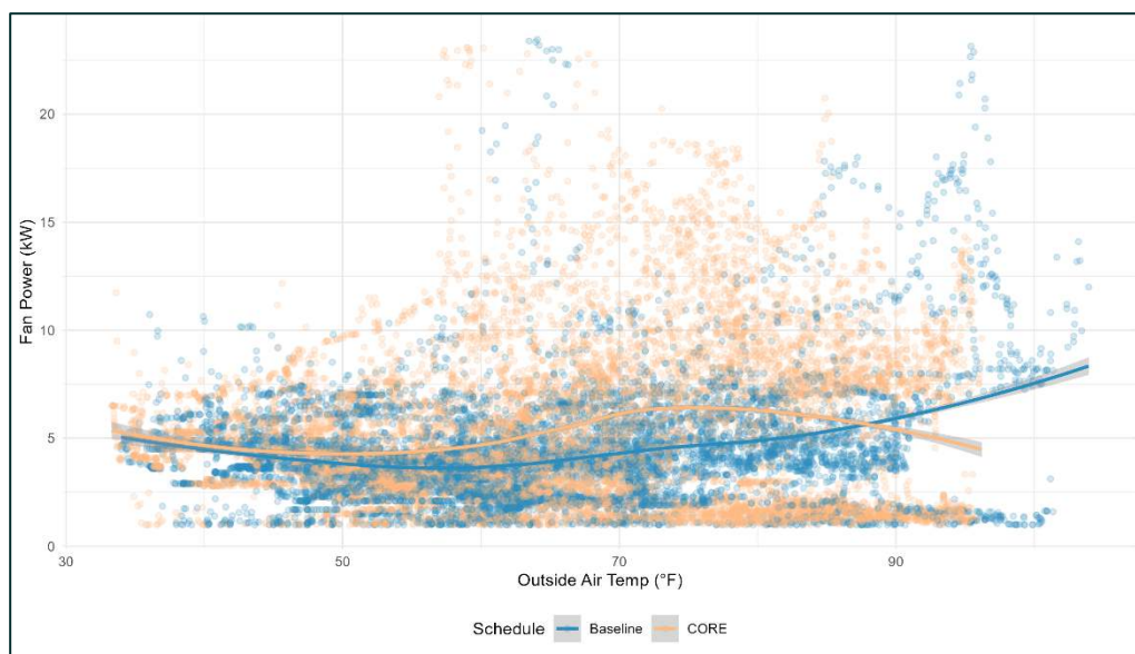
Figure 39: HVAC fan energy consumption vs. OAT for combined RTU 1 and RTU 2/3—MOB-2.
