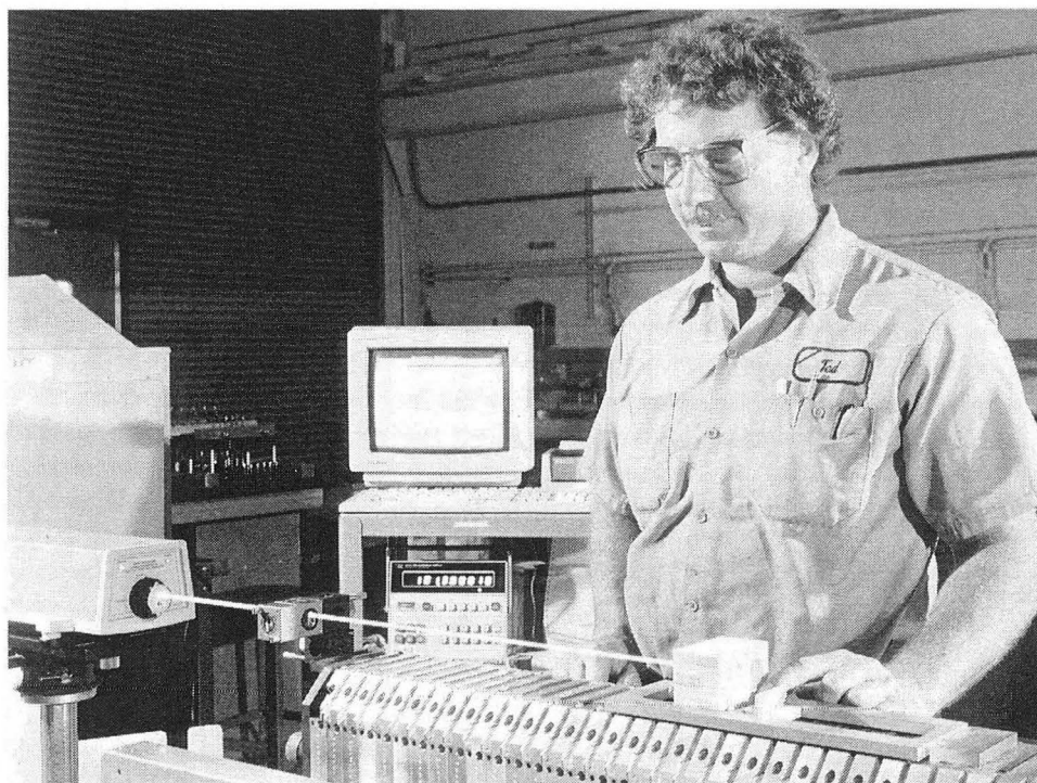
Figure 15. An assembly section undergoing alignment by a system employing a laser interferometer and computerized data acquisition.
