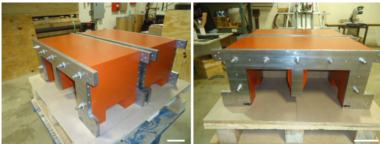
Figure 3.19: Photo of Assembled Iron Return Laminations. The iron return (in two halves) was assembled with C-5 coated, 16 gauge cold-rolled steel sheets. The epoxy-bonded laminations were then painted with a polyurethane varnish (orange) to prevent corrosion. Each half was then mechanically secured by custom stainless steel plates with electrically insulated bolts for structure support. Scale bars: 0.1 m.
