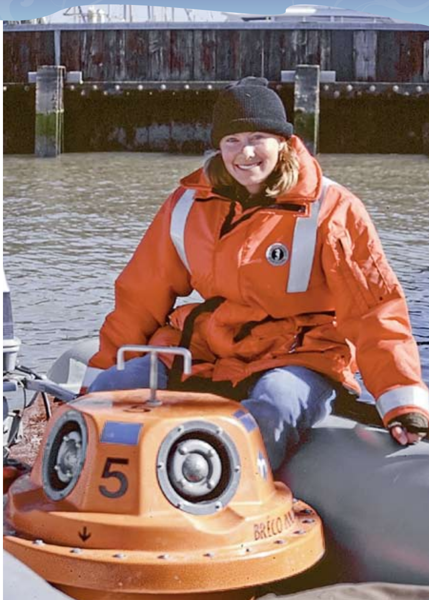
Figure 10. The Breco Bird Scarer is designed to float with a spill in all water conditions. Photo: D. A. Whisson.
