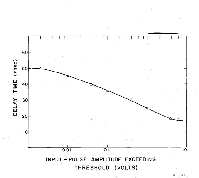
Fig. 4. Delay time for various increments of input-pulse amplitude above threshold.
