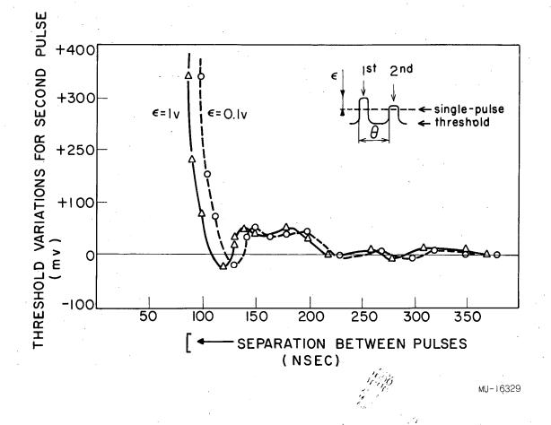
Fig. 3. Double-pulse resolution curves showing threshold variation vs. separation  $\theta$  between pulses.
