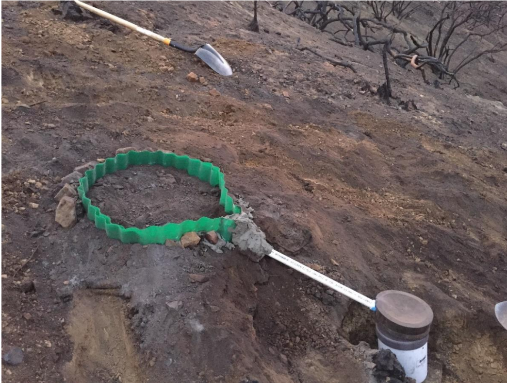
Figure A9. Small-scale runoff plot designed after Moody and Ebel (2012a) used to measure point-scale runoff production (location in Figure 1B). Runoff from the bounded plot is routed through a PVC pipe into a re-purposed tipping bucket gage with a mesh screen to prevent highly concentrated sediment from compromising tipping bucket measurements.
