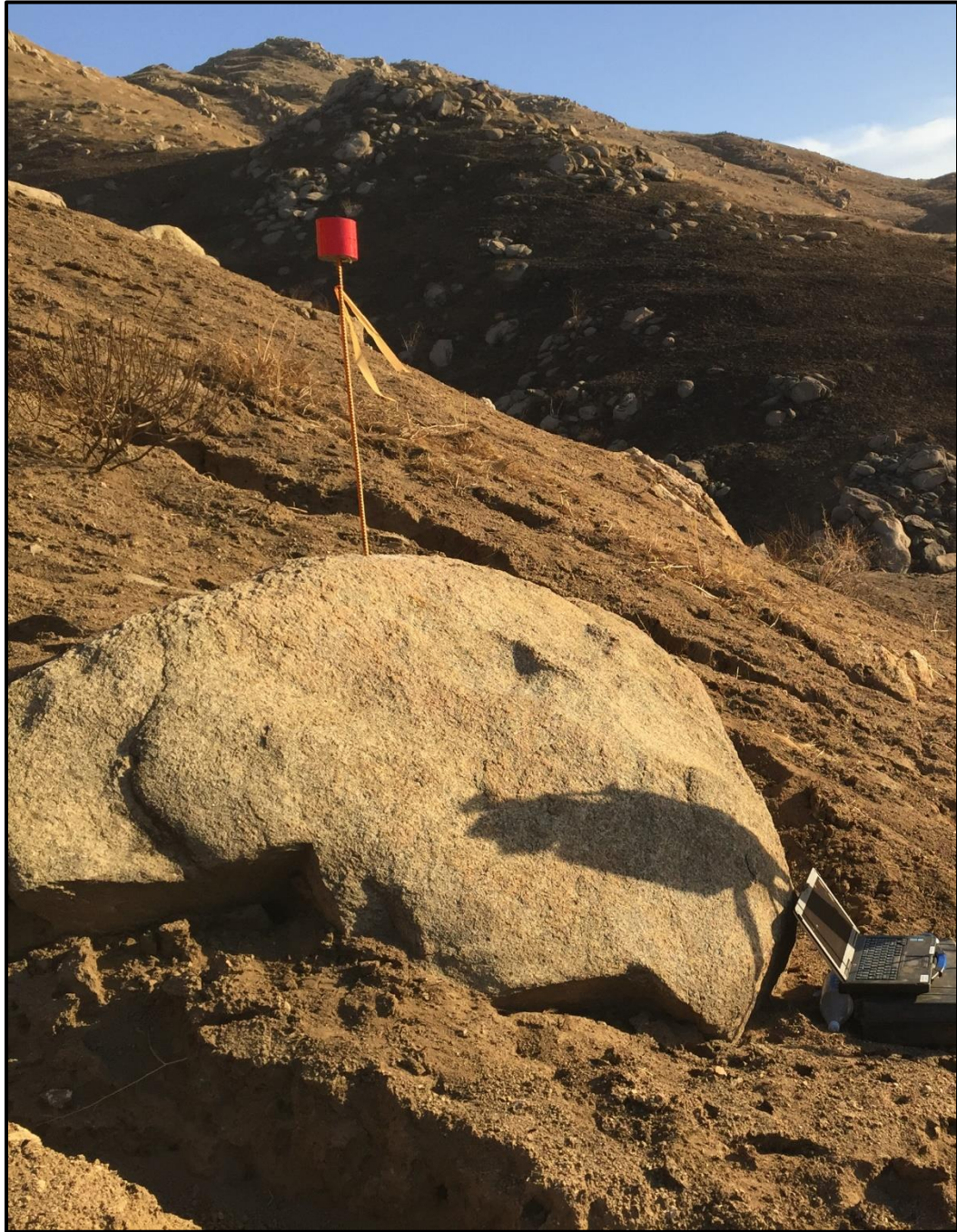
Figure A1. Picture of fixed cylindrical monument fixed on ½” rebar used as tiepoints used in this study. Laptop on the right shown for scale.
