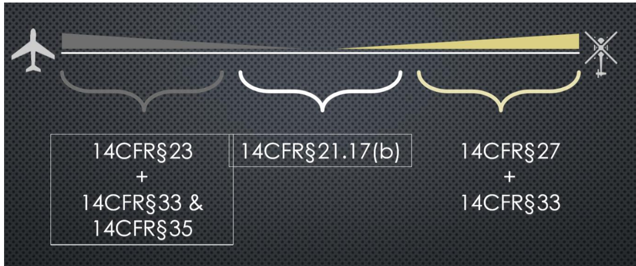
Figure 6: Range of certification approaches for hybrid fixed wing and rotary aircraft 38
