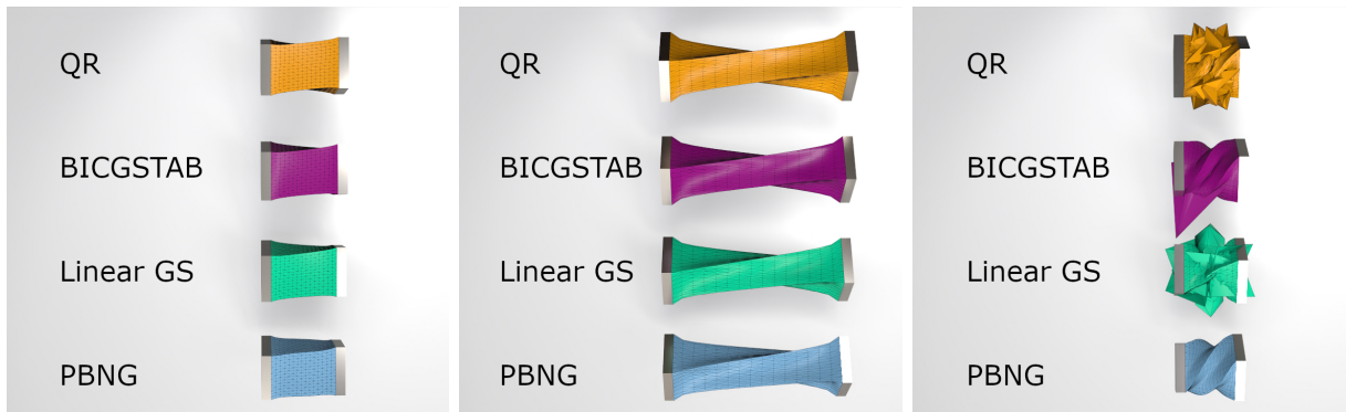
Figure 5.11: Hessian Comparison. The top three bars are simulated using Newton’s method with different linear solvers (QR, BICGSTAB and linear Gauss-Seidel respectively). The bottom bar is simulated using PBNG. The top bar uses the exact Hessian and becomes unstable. The bottom bar uses our Hessian projection and stays stable.
