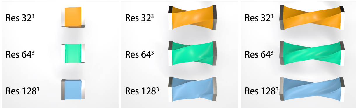
Figure 5.8: Different Mesh Resolution. PBNG produces consistent results when the mesh is spatially refined. The highest resolution mesh in this comparison has over 2M vertices and only requires 40 iterations to produce visually plausible results.
