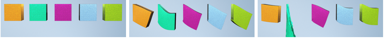
Figure 4.2: Equal Budget Comparison. From left to right: Newton (converged), Newton, FP-PXPBD, B-PXPBD, XPBD. With a limited budget, XPBD-style methods are stable, whereas the Newton’s method suffers from instability. Frame 0, 10, 60 are shown in the figure.
