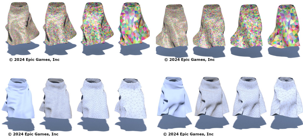
Figure 5.5: Multiresolution Dress. We illustrate the multiresolution meshes used with our MPBNG approach in a representative clothing simulation.
