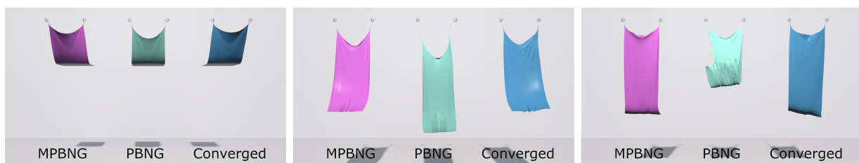
Figure 5.19: Draping Cloth . A piece of rectangular cloth with two corners clamped swings under gravity. With a fixed computational time of 1.8s/frame, MPBNG is much more similar to the converged look of the cloth than PBNG which appears too stretchy.
