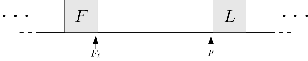
Figure 4.9: Here we depict the test to determine whether a run is pivotable . We define F and L as the first and last \lambda cells of the run. Our pivot p is the element just prior to L and F_\ell is the last element of F . This run is pivotable if F_\ell < p .
