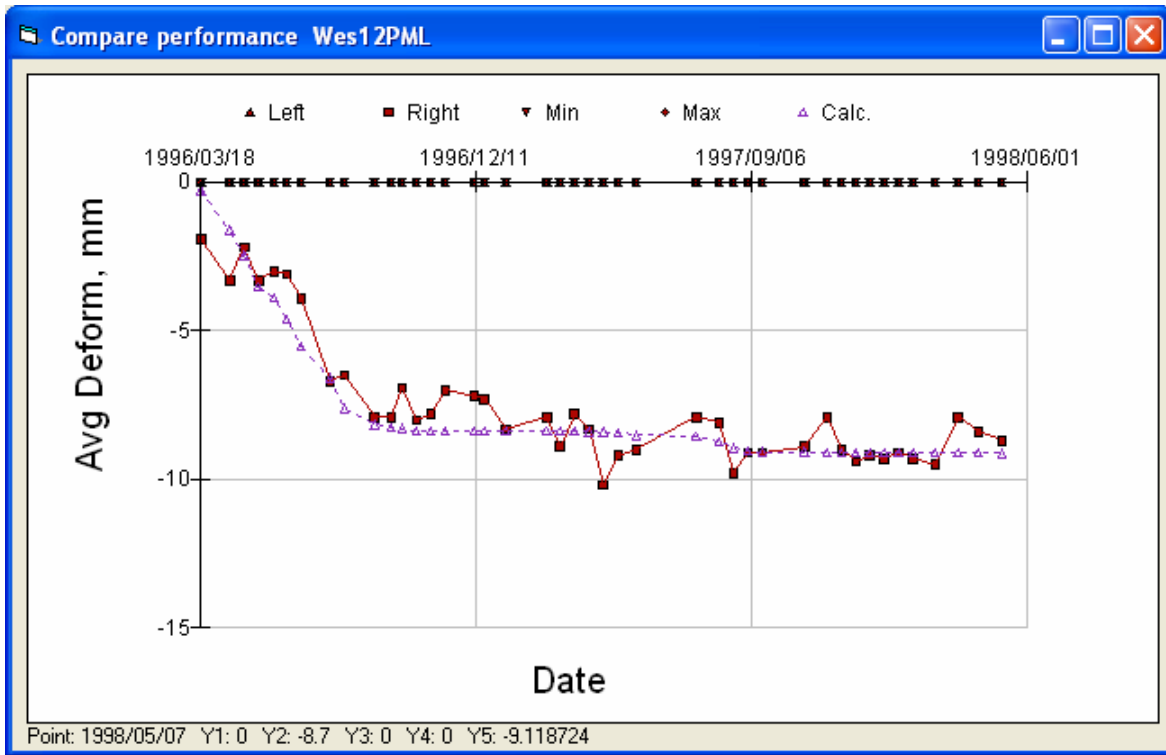
Figure 159. Down rut in right wheelpath at Section 12.
