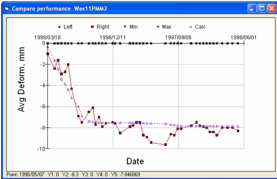
Figure 154. Down rut in right wheelpath at Section 11.
