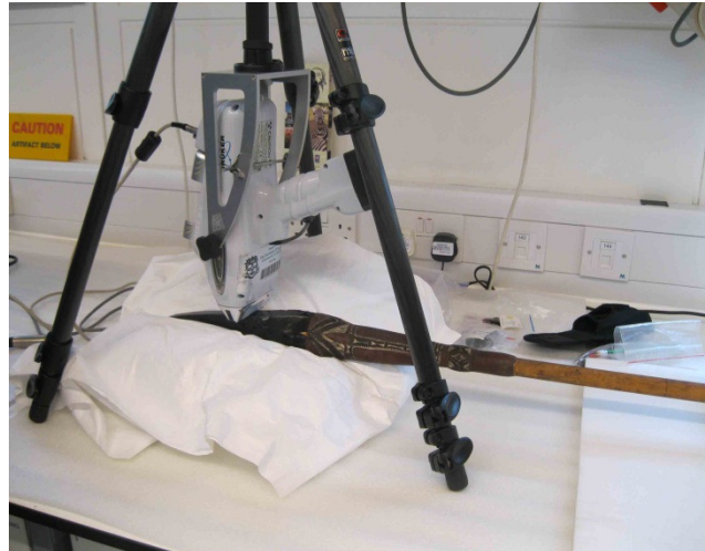
Figure 2. A typical obsidian-tipped blade with an incised gum haft (PR 1884.19.31) under analysis by PXRf at the Pitt Rivers Museum (photo by Robin Torrence by courtesy and copyright Pitt Rivers Museum, University of Oxford).
