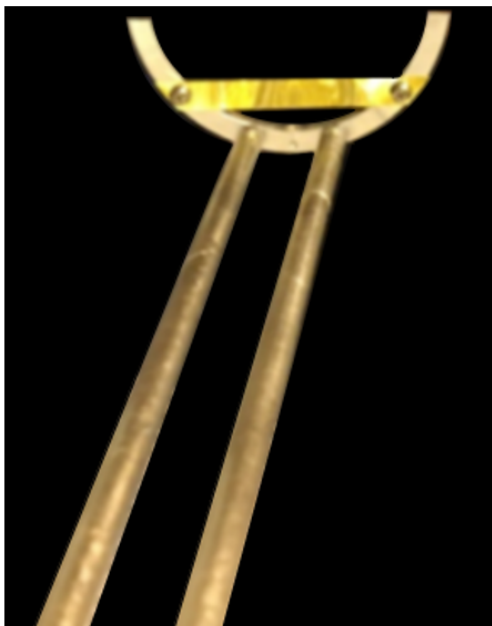
Figure 2.14. Fixed target apparatus including support beams, holding collar, and gold foil.
