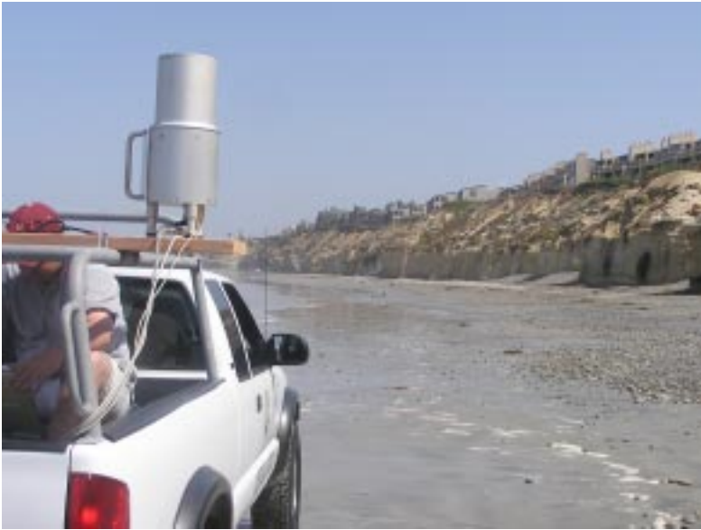
LIDAR scanning in process on a section of bluffs in Solana Beach. The laser emits infrared light and records its "echo." Photos this page: Christina S. Johnson, California Sea Grant
