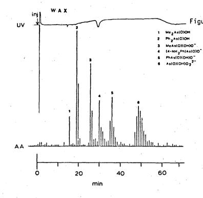
Figure 2. UV and arsenic-specific AA chromatograms for an aqueous solution containing five organoarsenic acids and arsenate (as numbered) are compared. Complete separations of this and similar mixtures of other arsenicals were effected in comparable analysis times.
