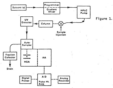
1. Schematic of HPLC-GFAA system showing programmed solvent gradient flow and in-line UV and GFAA detectors [5,28]. The GFAA spectrophotometer consists of a heated graphite atomizer (HGA) and an atomic absorption spectophotometer (AA).
