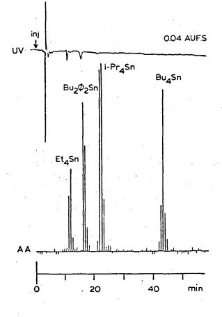
Figure 4. The isocratic separation of four tetraorganotins on an octadecylsilane chemically bonded phase columns, using methanol: H<sub>2</sub>O (93:7 vol.%) at a flow rate of 1.0 mL min<sup>-1</sup>.
