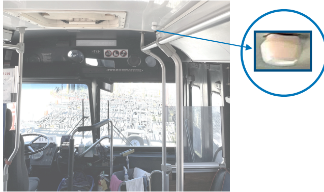
Figure 4.12: Example of placement of a BLE beacon (Kontakt Tough TB15-1) on the ceiling of the shuttle bus.
