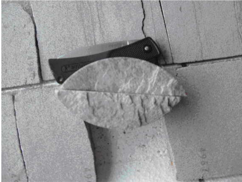
Opposing faces of a horizontal shear fracture
