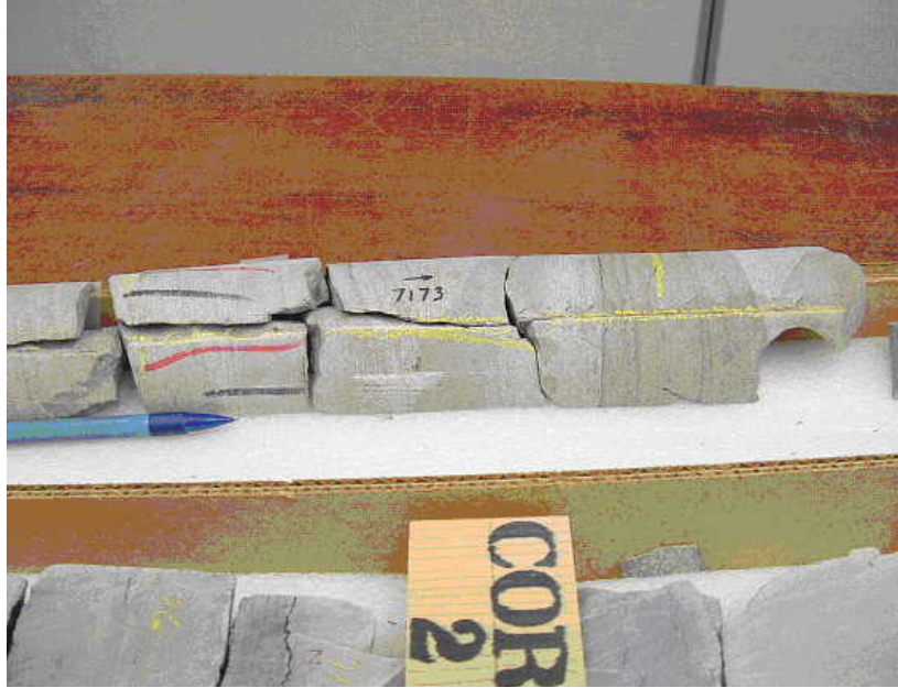
Scribe line, marked in yellow, that has imparted sufficient strain to the core to crack it. The induced fracture on the slabbed face resembles a natural fracture. San Juan 28-7 #238R
