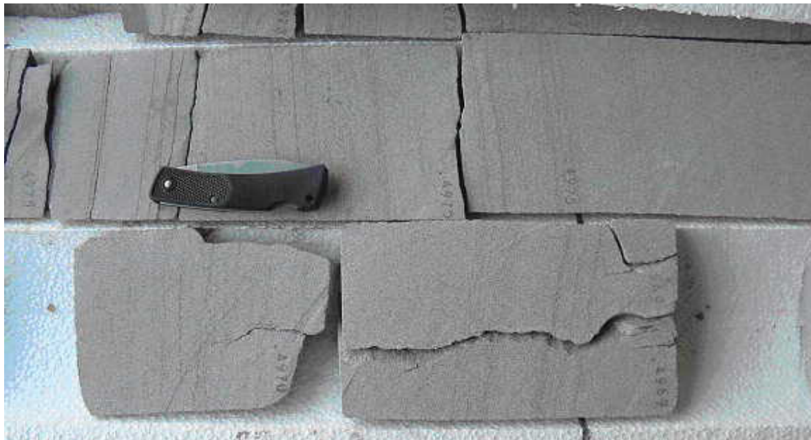
Two parallel vertical extension fractures. Apparent irregularity of the fracture plane is an artifact, accentuated by the narrow angle between the fracture plane and the plane of the slabbed face.
