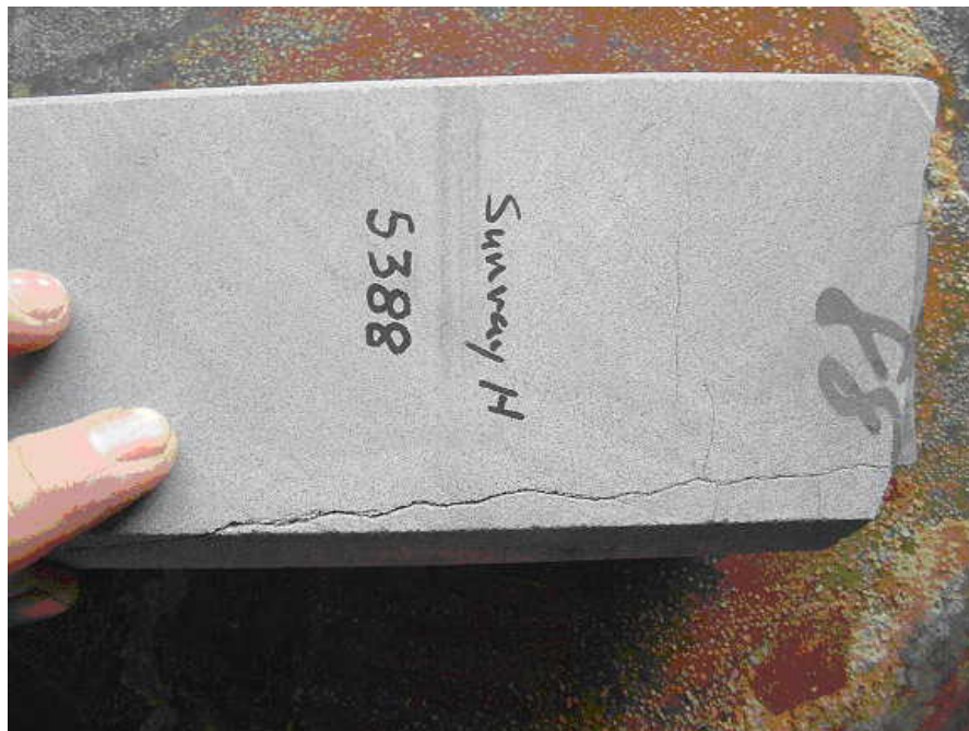
Open fracture aperture along the largest fracture noted in the core.
