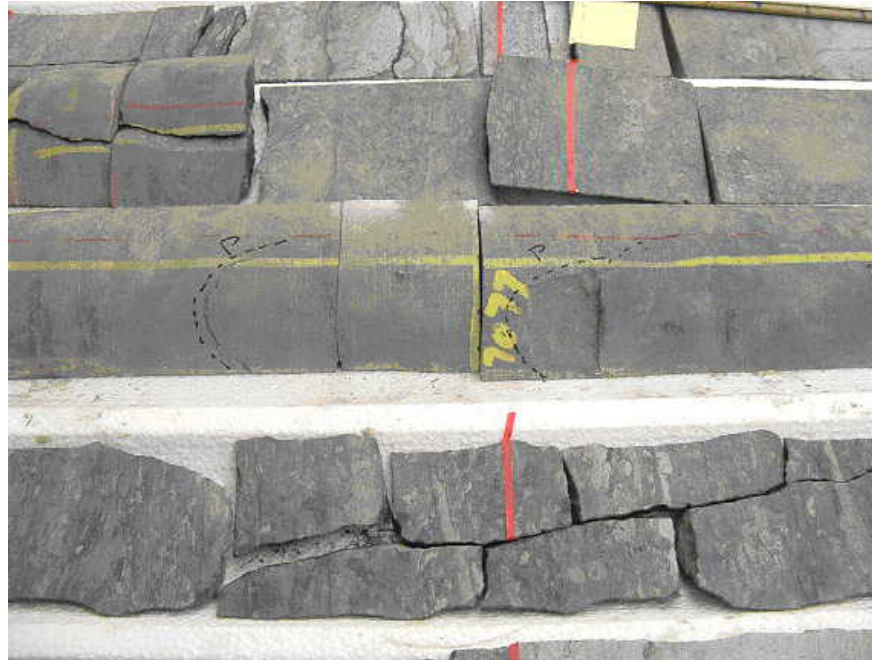
Parallel petal fractures (outlined in dotted black lines) and an inclined un-mineralized fracture, San Juan 28-7 #225E.
