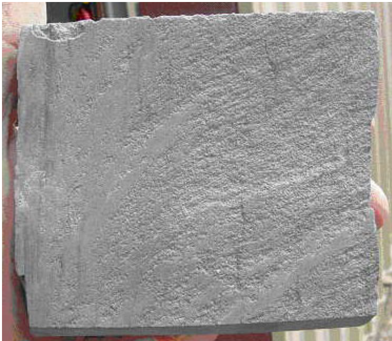
Plume structure on an unmineralized fracture face, indicating that the fracture formed in extension, not shear. The axis of the plume is horizontal (stratigraphic up is to the right), indicating that the fracture is natural.
