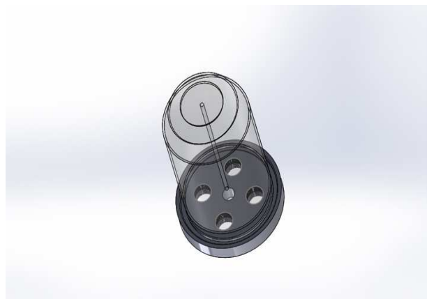
Figure 6.1 vacuum bonding chamber after assembly (left) and initial model of chamber area prepared by Solidworks
