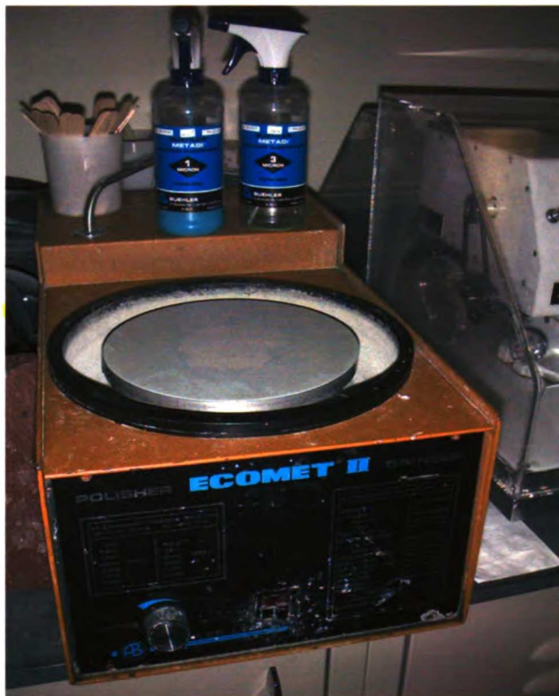
Figure 4. Buehler Ecomet II Polisher Grinder with Buehler Diamond Abrasives
