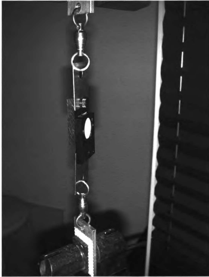
Figure 8. The single plane shear test assembly (SPSTA) affixed to the Instron Model 1122 Electromechanical Test System. Holding screws have been removed.
