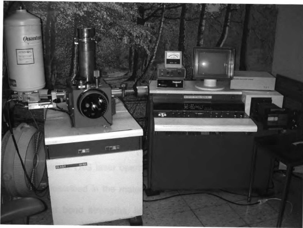
Figure 12. Topcon SX-40A "wet" environmental SEM
