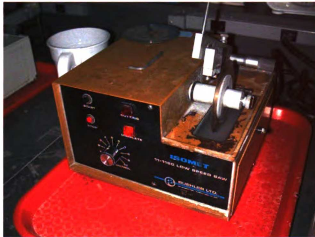
Figure 3. Buehler Isomet 11-1180 Low Speed Saw
