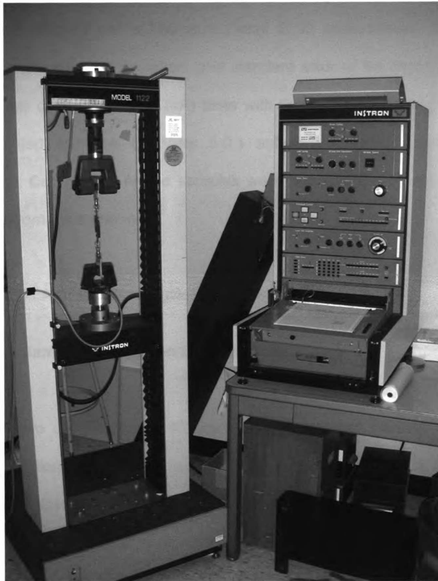
Figure 9. Instron Model 1122 Electromechanical Test System
