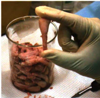
Figure 1. Harvested bovine incisors for use in sample preparation of 5x5 mm enamel blocks.
