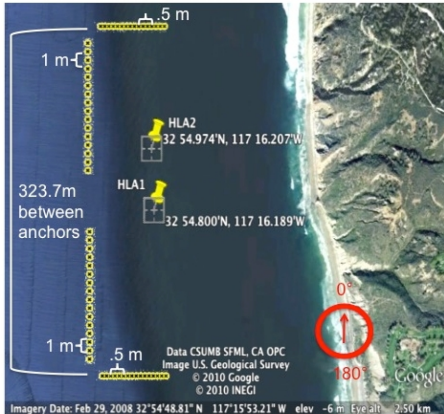
Figure 3.1: Experimental setup showing array shapes and location of anchors off the coast of San Diego, California. Each array is made up of 32 sensors set out in two perpendicular line arrays along the seafloor. The North-South line arrays (16 sensors on each array) have 1 meter spacing, the East-West line arrays (16 sensors on each array) have 0.5 meter spacing. The anchors (joining the two lines of each array) were 323.7 m apart. The water depth was approximately 20 meters throughout this region, and the measured sound speed profile was linearly uniform throughout the water column.
