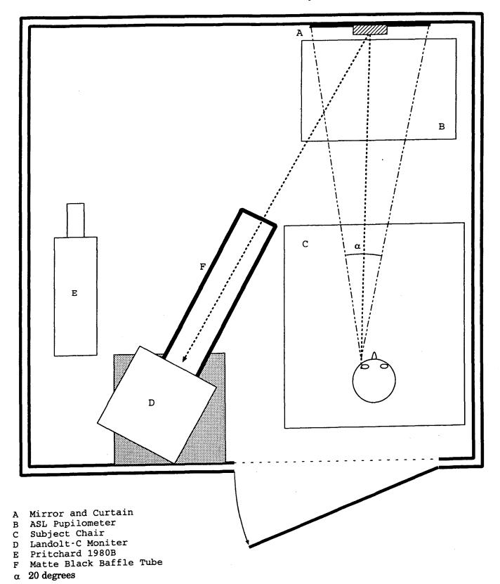
Figure 1: Layout of the aparatus used in our Landolt C experiments. The black curtain which surrounds the mirror subtends approximately 20 degrees and enables us to independly control the "surround" and the "task" lighting.
