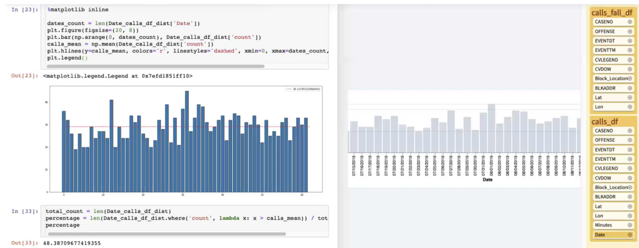
Figure 4.10: Using code to create a custom plot with the average line in the chart, and computing percentages.
