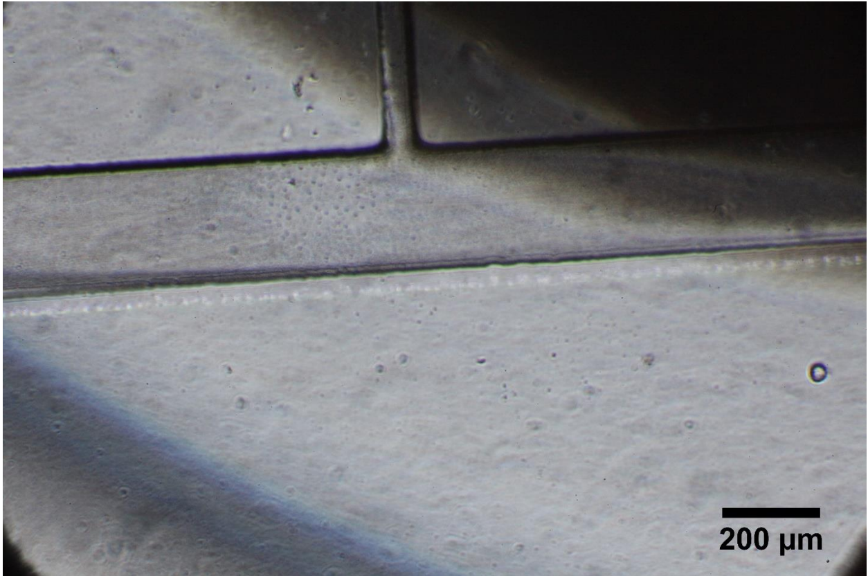
Figure 6: Run 4 was not primed with \text{CaCl}_2 , and blood was able to travel within the main channel along a distance of approximately 5mm
