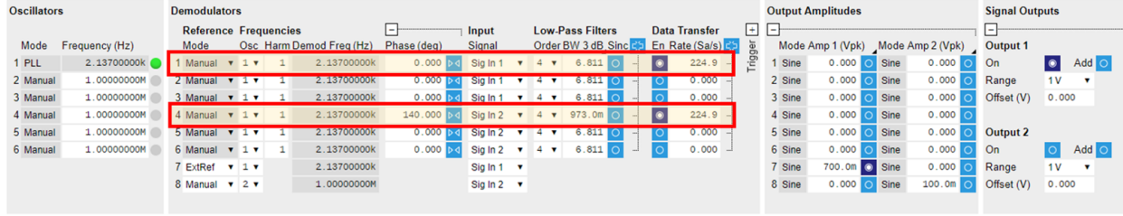
Figure G.54: User interface software configuration to extract the output of the CVG device under the test
