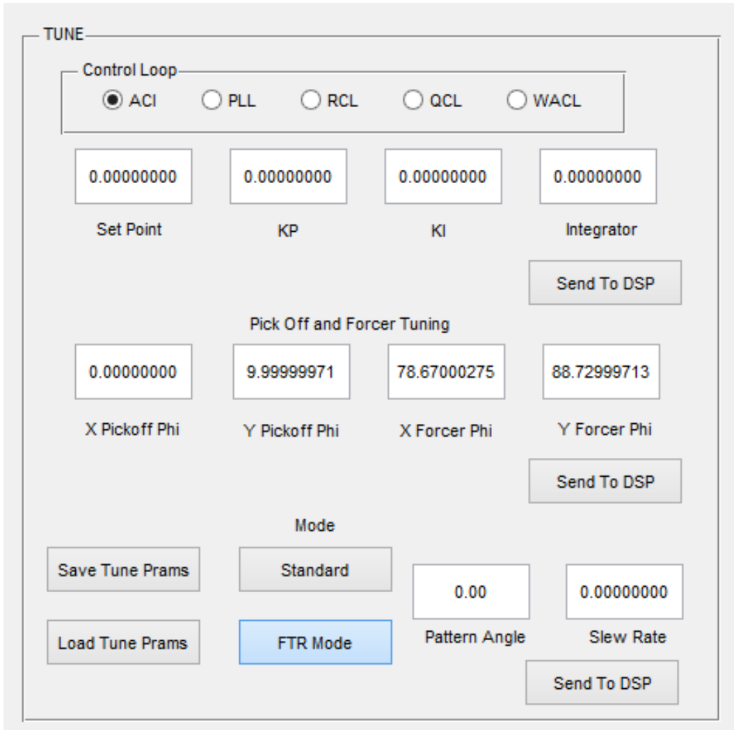
Figure H.61: PID tune-up GUI. Send/set parameters of each loop to the CODEC. Main loops are: Amplitude, Phase, Rate, Quadrature and Angle. Set drive forcer and pickoff phases.
