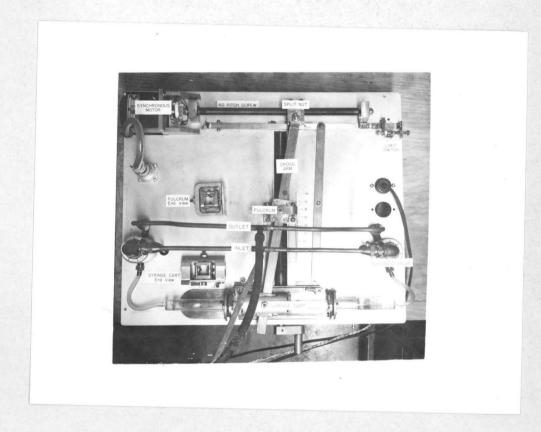
Fig. 1. Positive-feed, variable-flow-rate fluid pump (from above).
