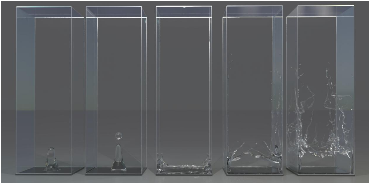
Figure 5.9: Spherical Drops. Spherical droplets with different surface tension coefficients free fall from the same height. In the top figure, from left to right, the surface tension coefficients are k^\sigma = 20, 5, 1, 0.1, 0.05\text{N/m} .
