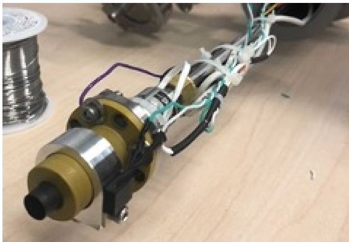
Figure 7.6: Pulsed discharge design for radical production. Precursor sample in the gas-phase is being introduced through a Parker 9 series valve, which passes through a copper disc that is electrically insulated from the rest of the valve. The copper disc is connected to a DC voltage supply and can operate up to 2000 V in both polarities.
