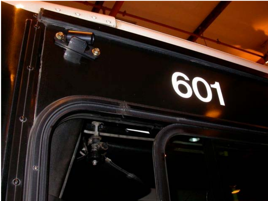
Figure 2-7 - Left Side Camera on SamTrans Bus 601
