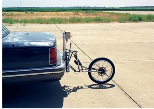
(b) Fifth wheel for target vehicle speed measurement
