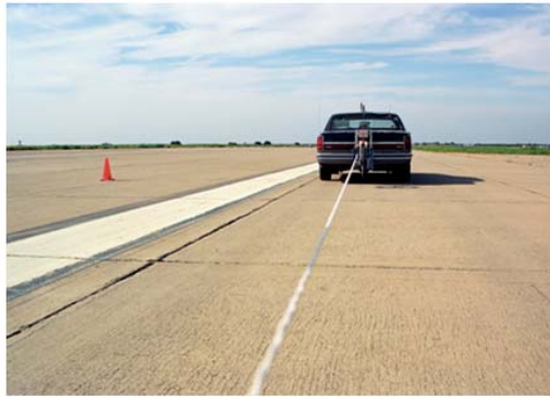
(c) String pot for target vehicle distance measurement
