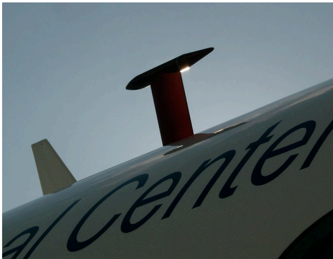
Figure A1-07. The MEDUSA HIMIL seen atop the GV fuselage during the HIPPO campaign. Air passed from right to left in the image, entering the small aperture at the front of the red HIMIL. MEDUSA air was picked off from the rear-facing inlet to avoid the introduction of moisture to the sample line. Photograph: B. Stephens.
