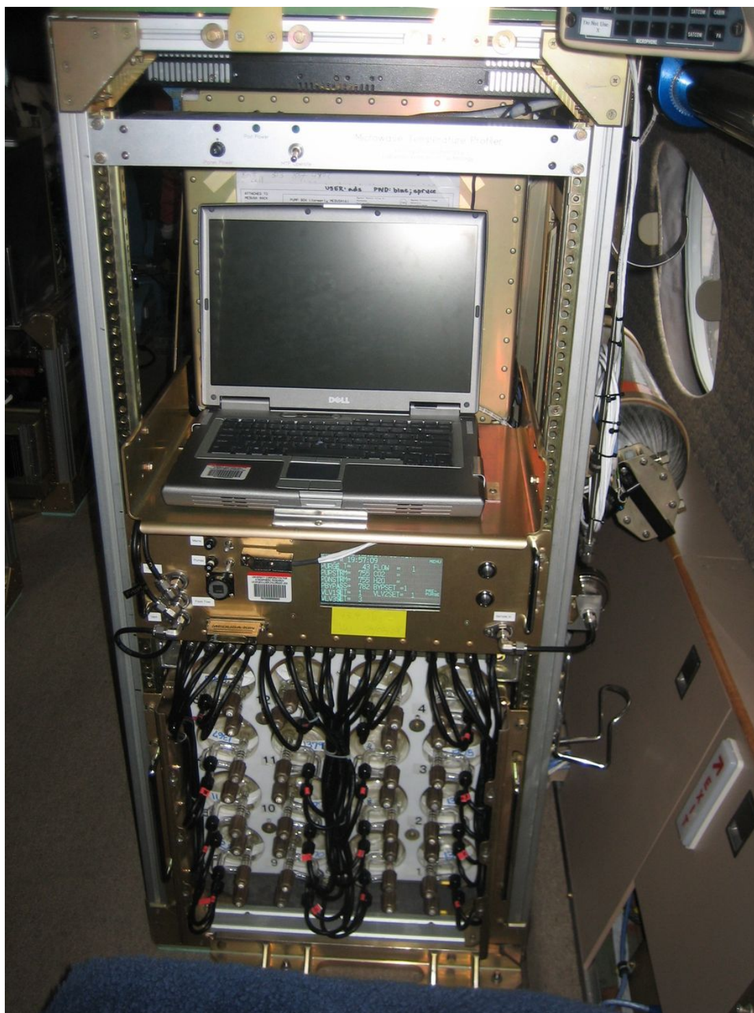
Figure 2.2. The front of the MEDUSA sampler, as seen by the operator, showing a laptop workstation (not part of MEDUSA), the pump box beneath it (gold color) and Flask Box 1 near the floor, with splinter shield removed to show the arrangement of the flasks.
