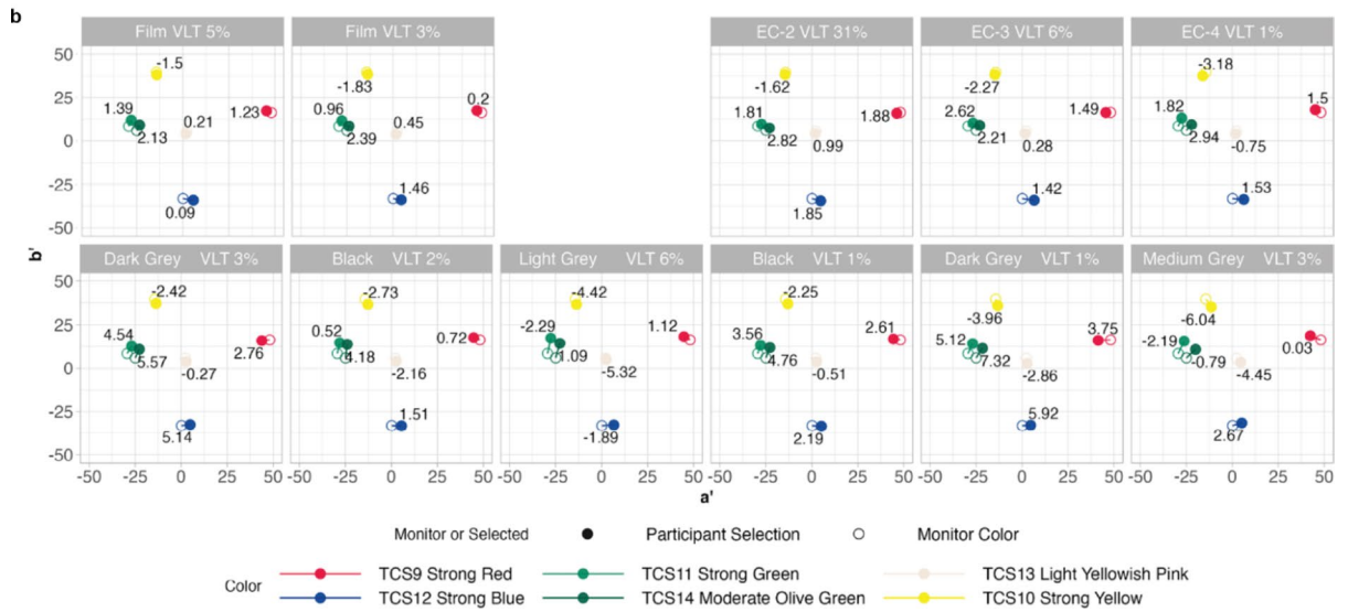
Figure 3. (a) Effect of window films, electrochromic glass, and fabric shades on participant ability to match TCS9–14 colors. Color matching accuracy represented by Euclidian distance ( \Delta E ) in the CAM16 color space between actual color and participant selection. Mean of the scores and the standard error of the mean bars; (b) Effect of window films, electrochromic glass, and fabric shades on participant ability to match the hue of TCS9–14 colors. Hue shift is represented as the hue distance ( \Delta a'b' ) between TCS9–14 swatches and the mean participant color selection in CAM16 color space. Lightness shift ( \Delta J' ) is listed as a numeric label next to the corresponding points. The visualization method is adapted from 22 .
