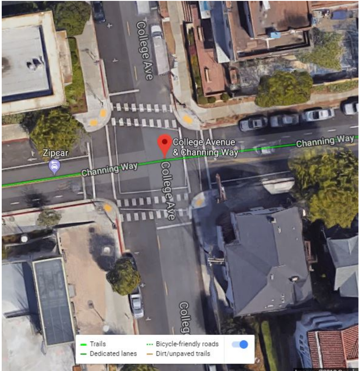
Figure 2.25: Sample intersection with 4 approaches and at least 1 left-turn lane
