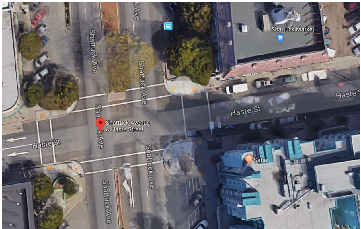
Figure 2.29: Sample intersection with 3 approaches and at least 1 left-turn lane
