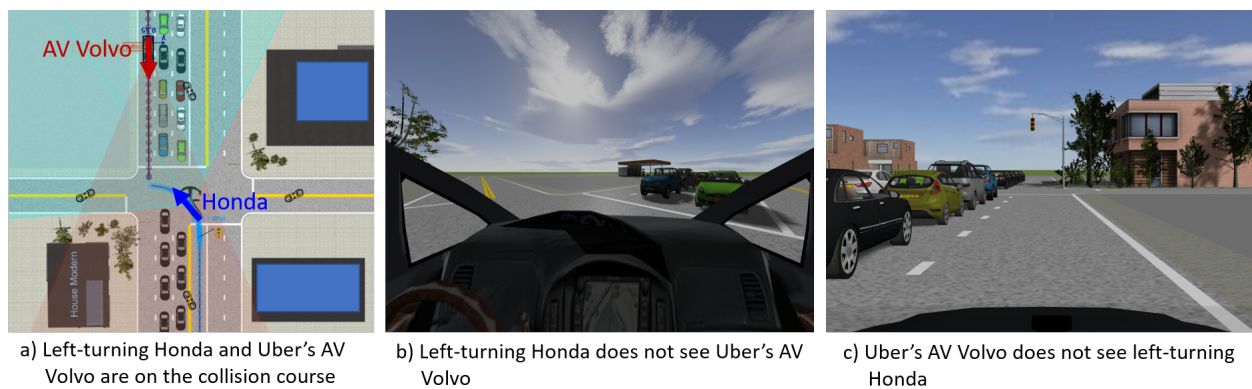
Figure 2.2: PreScan simulation of V_1 and V_2 collision — snapshot of the scenario 2 seconds before the accident.
