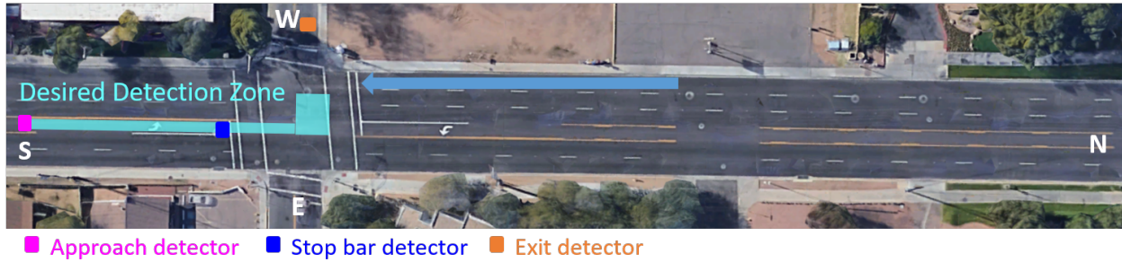
Figure 2.17: Desired detection for the north-to-south through movement.
