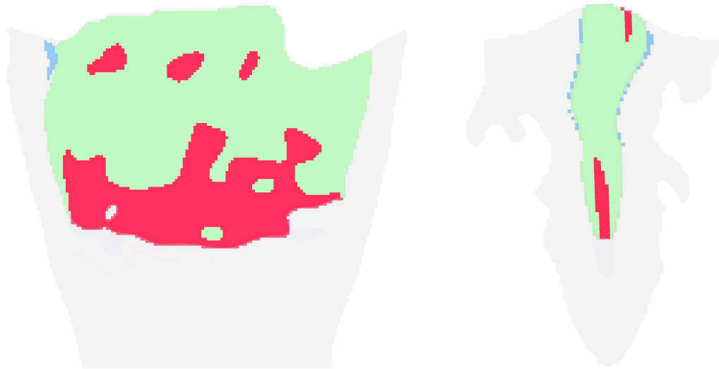
Figure 5.9: Slices oriented along the X (left) and Y (right) axis of the segmented regions of the Methane dataset. Here segments for pressure (blue), temperature (green), and CO_2 (red) are depicted only for high distribution values. Grey regions indicate areas of lower distribution values in the query’s solution set.
