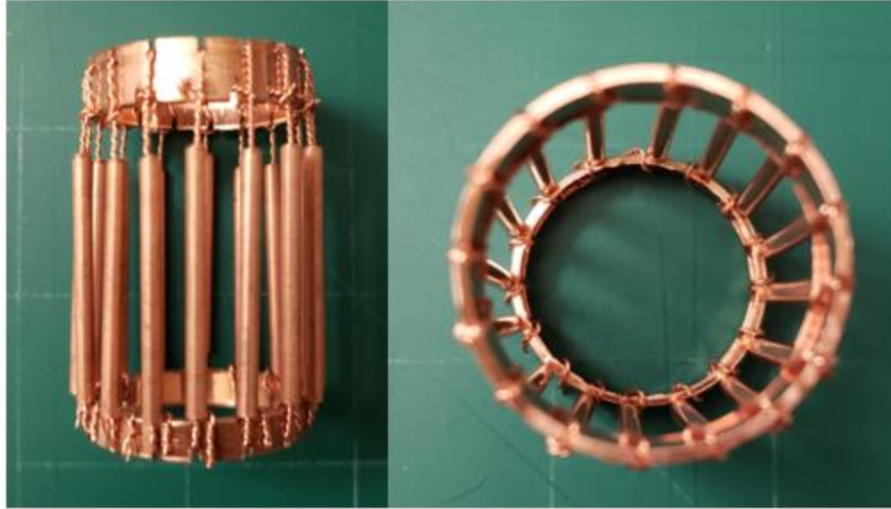
Figure 4.1 Side and Top view of a completed CFC made with bare copper tubes of 2.38mm diameter secured to the holders with twisted copper wires.
