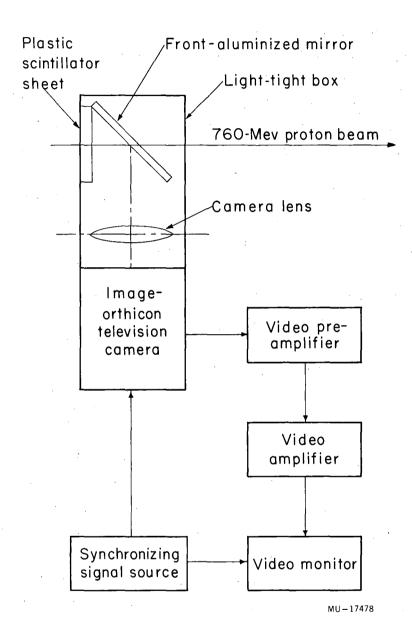
Fig. 1. Block diagram of basic camera chain.
