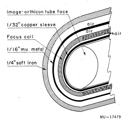
Fig. 2. Image-orthicon shielding arrangement.
