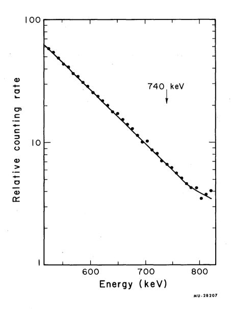
Fig. 6. Scintillation spectrum observed in decay of Pr<sup>143</sup> plotted on a semi-log scale so that background due to bremstrahlung will be linear.
