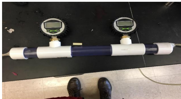
Figure 2-6. Benchtop Assembly for Stent Occlusion Diagnosis.
