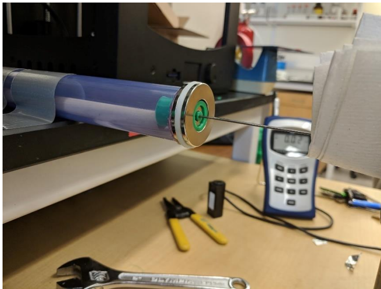
Figure 6-4. Benchtop Set up for the Magnetic Shielding Experiment.
