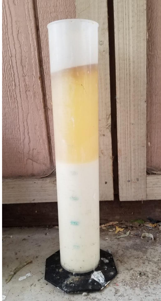
Figure 13: Biomineral production is quantified using a graduated cylinder, whereby the settled volume represents the biomineral formed in the sedimentation tank in a week's time.
