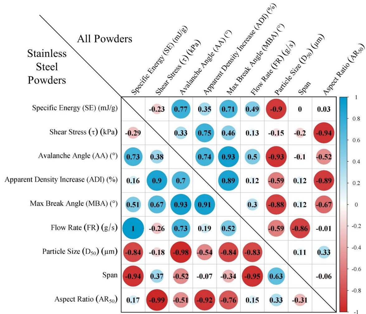
Figure 2.2. R-values correlating parameters used in this study. The lower left of the matrix displays R-values for stainless steel powders, while the upper right is for all powders. The size of the circles shows the intensity of the correlation, while the positive /negative numbers and the blue/red colors indicate direct/inverse correlations, respectively.
