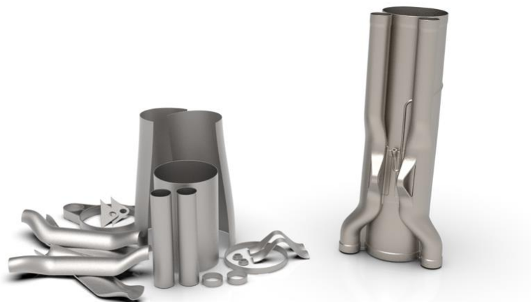
Figure 1.1. a) design used in conventional manufacturing consisting of many smaller parts; b) design used in AM consisting of one part [2].
