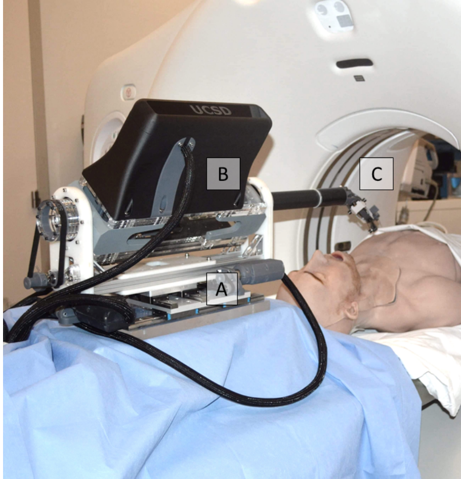
Figure 2.1: CT-guided robotic system with a low-intra-bore-profile serial-link redundant 7-DoF arm. A is the cartesian positioning stage. B is the trunnion and rotary axis. C is the robotic 4DoF arm.
