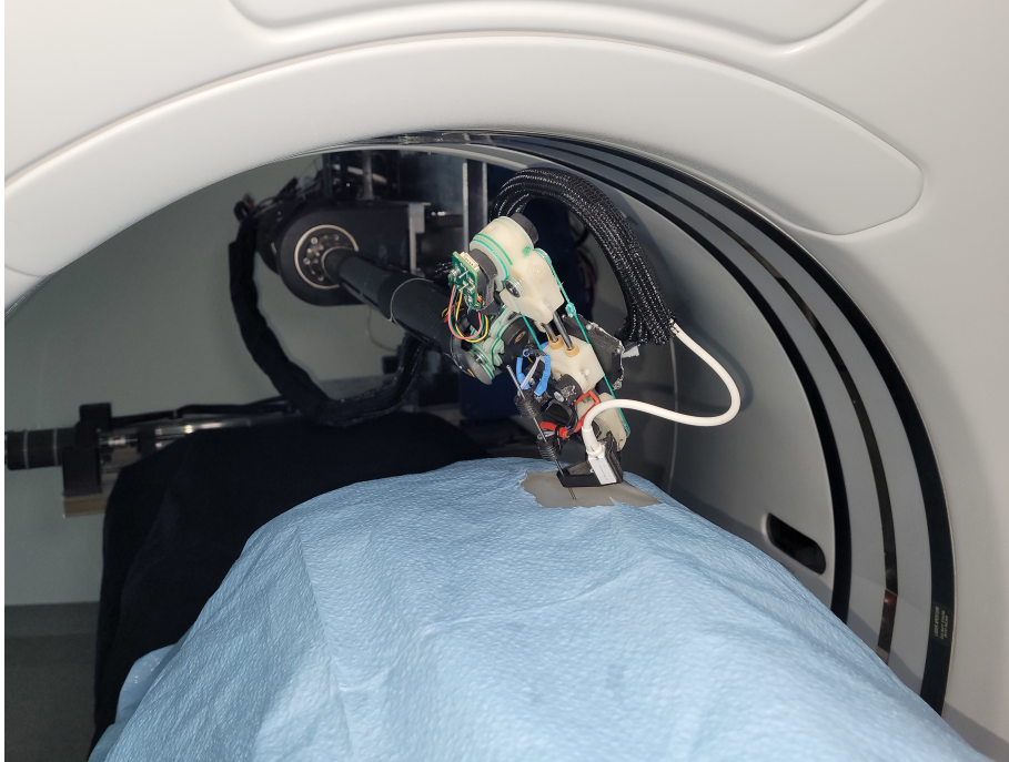
Figure 3.1: Needle insertion within imaging bores provides direct volumetric visualization of the anatomy and tool, improving the accuracy of needle insertion procedures such as retroperitoneal biopsy and lumbosacral spine nerve block. However, this enclosed environment limits the space for manipulation and line-of-site visibility for devices. CRANE overcomes these challenges with its cable-driven serial link design and integrated planning-control method to enable fully in-bore dexterous needle manipulation without requiring manual setup.
