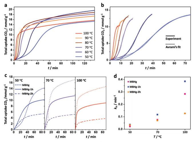
**Figure 5.** a)  $CO_2$  reaction kinetics in pristine MBHg at various temperatures from a 15%  $CO_2$  in N<sub>2</sub> stream. b) Avrami's fractional-order kinetic model of the experimental  $CO_2$  uptake profiles presented in (a). c) Comparison of the gravimetric  $CO_2$  uptake in MBHg, MBHg-1h, and MBHg-2h at three temperatures from a 15%  $CO_2$  in N<sub>2</sub> stream. d) Avrami rate constant ( $k_A$ ) as a function of temperature for MBHg, MBHg-1h, and MBHg-2h.
