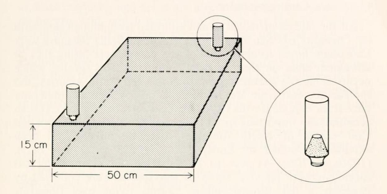
Figure 1. Schematic Diagram of Emergence Trap Showing Positions of Two Screw-Cap Vials in Situ. Each Vial Has a Plastic Cone Glued Into the Opening.
