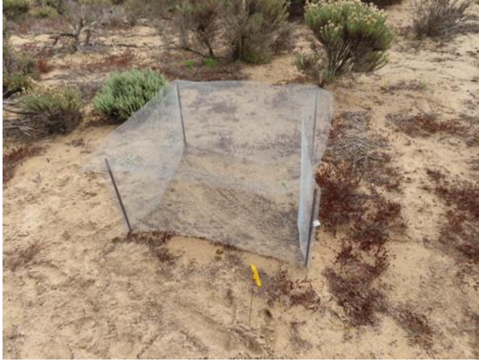
Figure 3b. Fully caged to collect fog and prevent herbivory.
