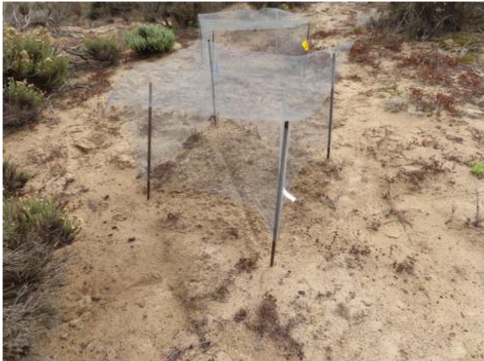
Figure 3a. Raised cage. Collects fog and allows for herbivory.
