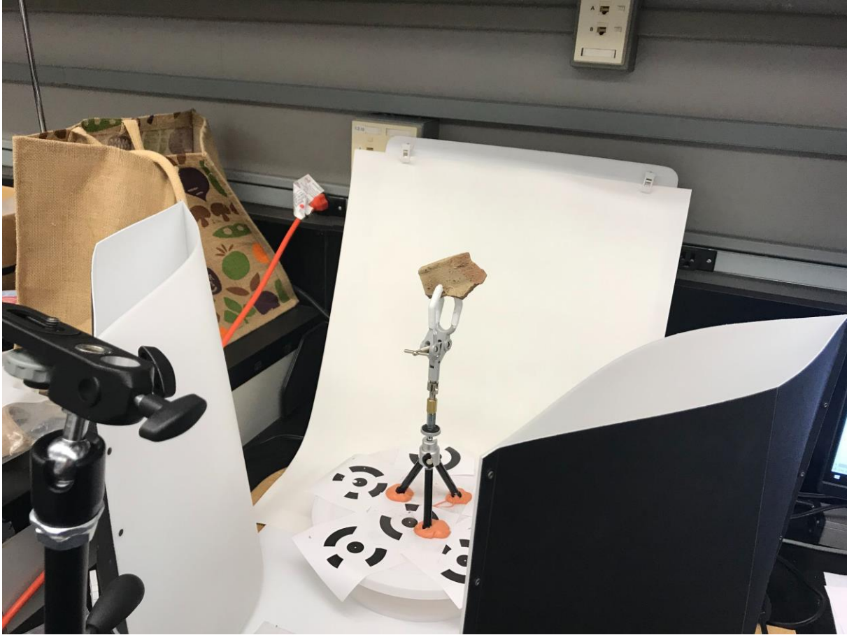
Figure 8.1: A view of the IBM rig. At left is the Manfrotto Magic Arm, which holds the camera while the rig is in use. At left and right are two lightboxes that provide indirect light to the front of the sherd. At center is the custom tripod/clamp, holding a sherd from KAJ, placed atop a rotating cake stand. At the back of the image is a customizable backdrop.
