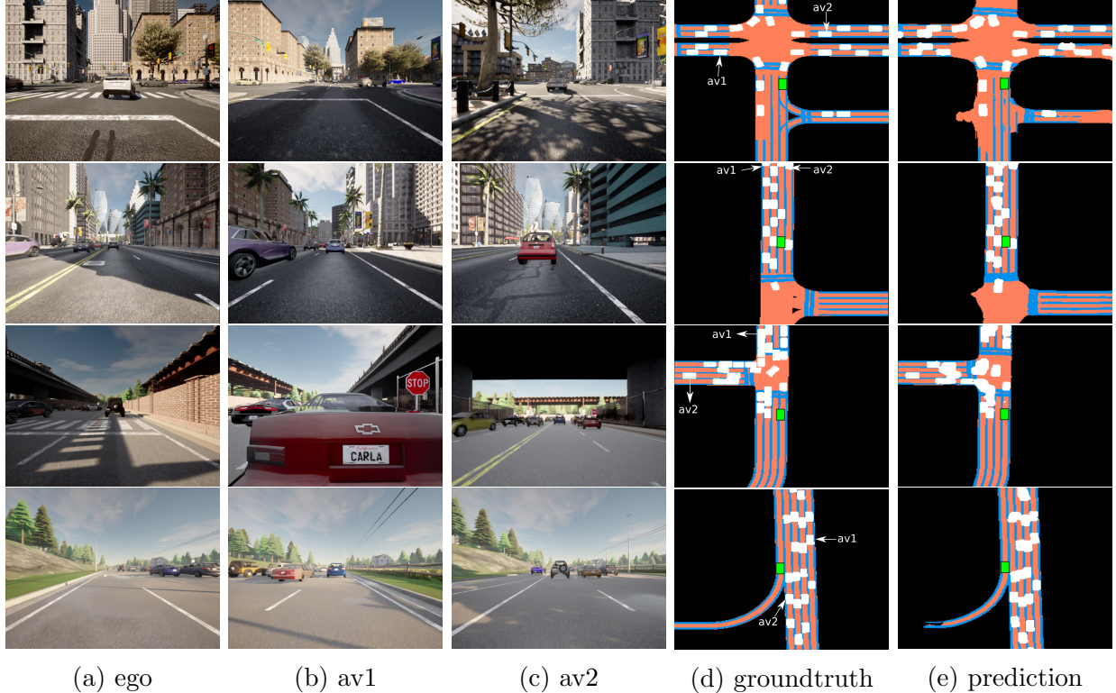
Figure 5.4: Qualitative results of CoBEVT. From left to right: the front camera image of (a) ego, (b) av1, (c) av2, (d) groundtruth and (e) prediction. The green bounding boxes represent ego vehicles, while the white boxes denote the segmented vehicles. CoBEVT demonstrates robust performance under various traffic situations and road types. It is also capable of detecting occluded or distant vehicles (white circled) benefiting from the collaboration.
