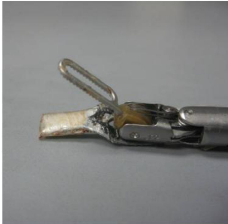
Figure 1. Waterproof sensor mounted on da Vinci robotic instrument
