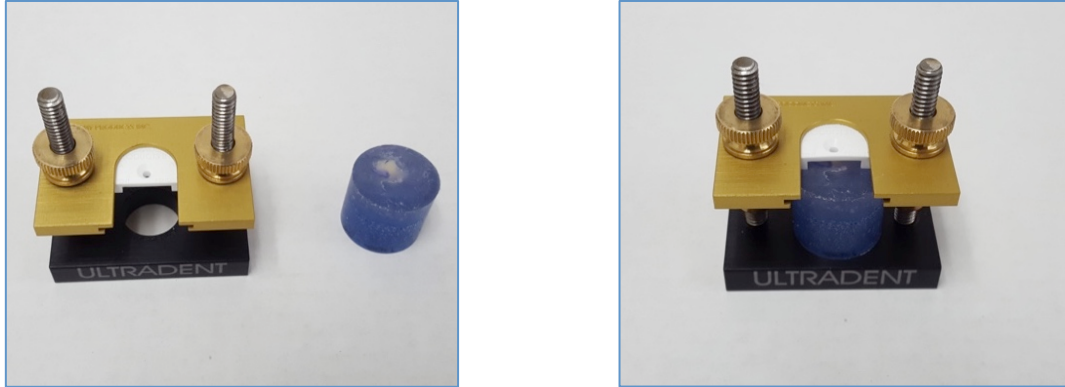
Figure 9: Ultradent Bonding Clamp and Mold Insert
