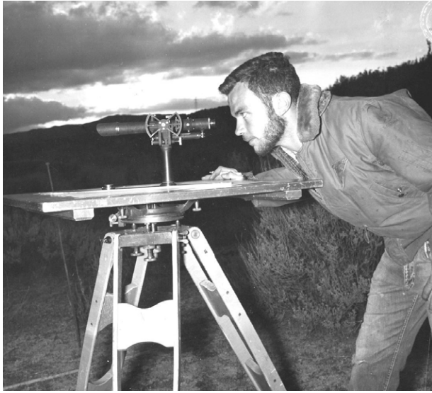
Figure 22.3. Mike using a plane table at a site in the San Bernardino Mountains, California, when he was a sophomore at the University of Redlands. (Courtesy of Michael E. Moseley.)
